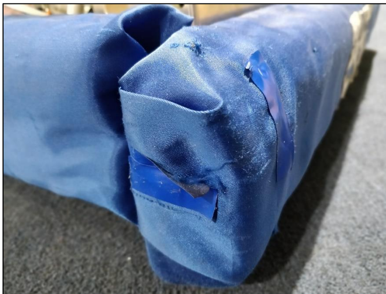
Figure 11: Bumper with tape covering ripped areas.
