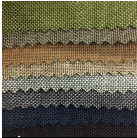
Figure 3: 1000 Denier Coated Cordura® Nylon Fabric
