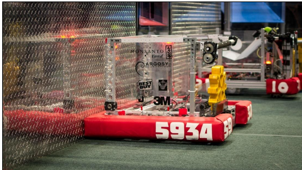
Figure 2: Team #5934 with Sail Cloth bumpers. One piece method with angled corners.
