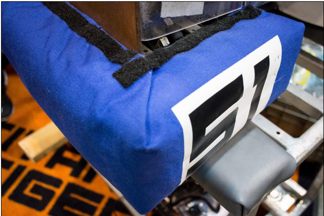
Figure 10: Bumpers with Velcro attaching cover.
